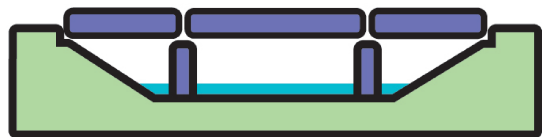
Beam Bridges go straight across.
