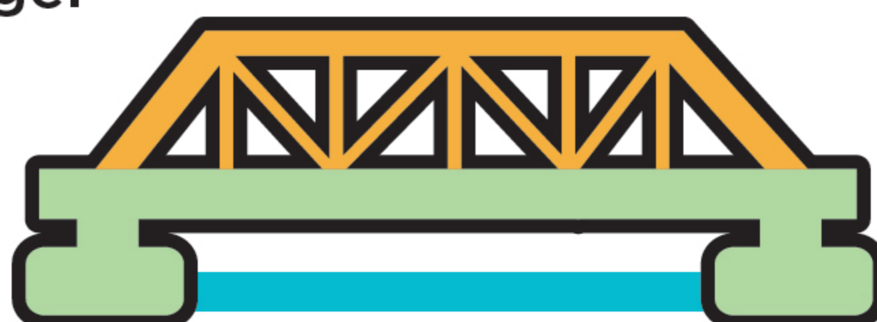
Truss Bridges use triangles to spread the weight.
